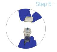
Open the sealed tube, which contains the sterile mini tube.
