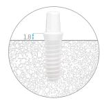
Implantation is completed when the implant is positioned 1.8mm above the bone level.
